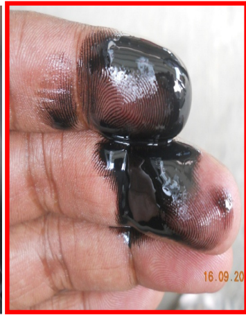
Oil (turning black ) after running few hours
