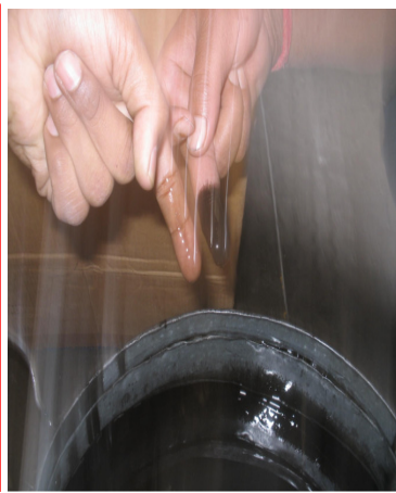
Oil (turning black ) after running few hours
